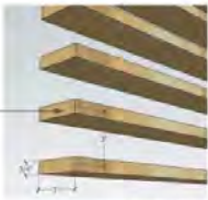
Wood Slat Wall Detail
